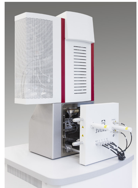
▲ Fig. 1: The Gatan 3View2XP ultra-microtome integrated in TESCAN MAIA3 XMU SEM.
